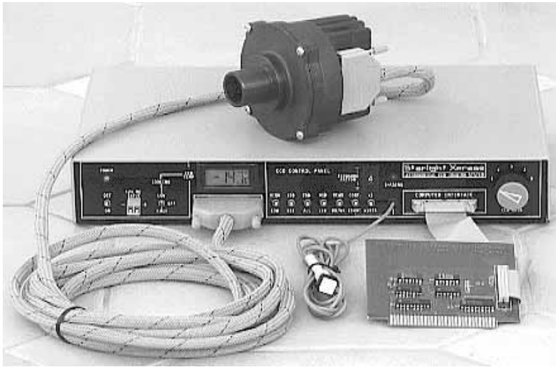
Figure 5.2 The Starlight Xpress SFX system is unusual in that it can capture and display images without the need for a computer. Saving and processing images does, though, require a computer.
