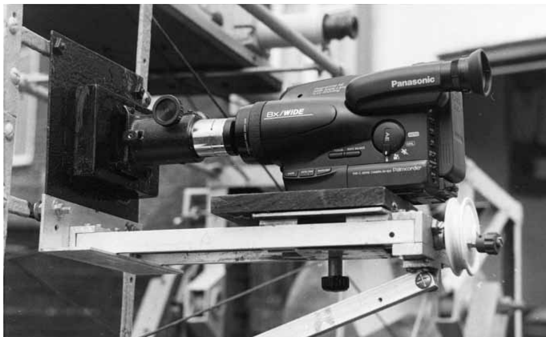
Figure 5.7 The arrangement the author uses to attach his video camera to his telescope. Counterweights (not shown) attach to the bottom end of the telescope tube to restore the balance.
