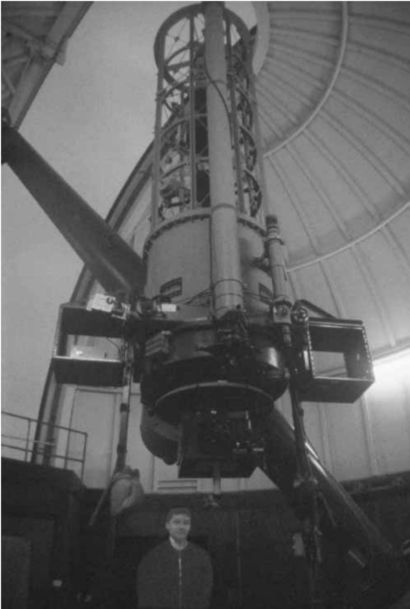
Figure 9.2 The author can be seen below the 36-inch (0.91 m) Cassegrain reflector at the Herstmonceux site of the former Royal Greenwich Observatory.
