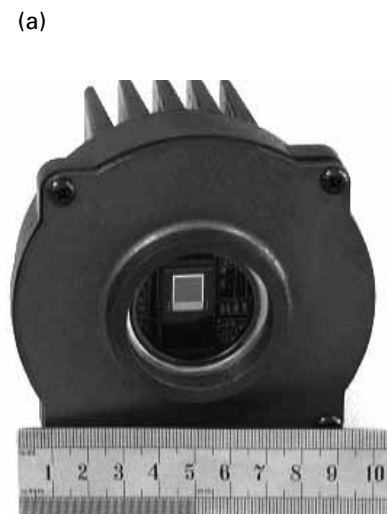
Figure 5.1 (a) The Starlight Xpress SXL8 camera head. The CCD can be seen within it. (The scale is in cms.) (b) The complete Starlight Xpress SX camera system, typical of commercial units.
