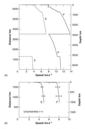
**Figure 4.9** Seismic wave speeds in (a) the Earth and (b) the Moon (global averages).
