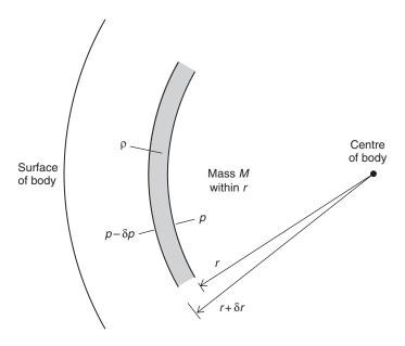
**Figure 4.10** The balance of forces on a spherical shell in a planetary interior.
