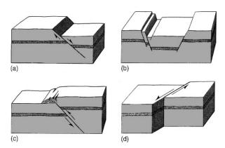
**Figure 6.6** Three kinds of fault. (a) A normal fault. (b) A graben (rift valley), made up of two normal faults. (c) A thrust fault. (d) A strike–slip fault. (From *Moons and Planets, An Introduction to Planetary Science* 3rd Edition, by Hartmann, 1993, Reprinted with permission of Brooks/Cole, a division of Thomson Learning: www.thomson rights.com, Fax 800 730–2215)
