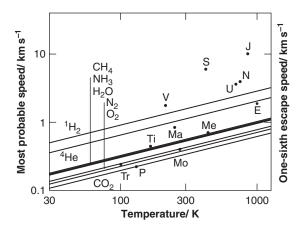
Figure 9.12 The most probable speed  $v_{\rm mps}$  versus temperature T for some major atmospheric gases. Planetary bodies are at the temperatures at the base of their exospheres.
