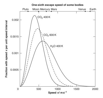
Figure 9.11 The Maxwell distribution of speeds of CO<sub>2</sub> and H<sub>2</sub>O, compared with one-sixth of the escape speed of some planetary bodies.
