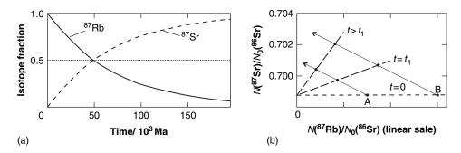
**Figure 3.15** (a) The principle of radiometric dating using the decay of <sup>87</sup>Rb into <sup>87</sup>Sr. (b) The Rb–Sr isochron plot for two minerals, A and B. The dashed lines are isochrons at three different times.
