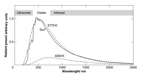
**Figure 1.1** The solar spectrum, and the spectra of ideal thermal sources at  $5770 \,\mathrm{K}$  and  $4000 \,\mathrm{K}$  (1 nm =  $10^{-9} \,\mathrm{m}$ ).
