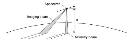
**Figure 6.1** Pulse altimetry and synthetic aperture radar.
