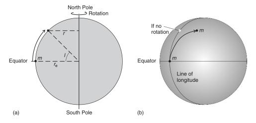
**Figure 9.14** The Coriolis effect at a planetary surface.
