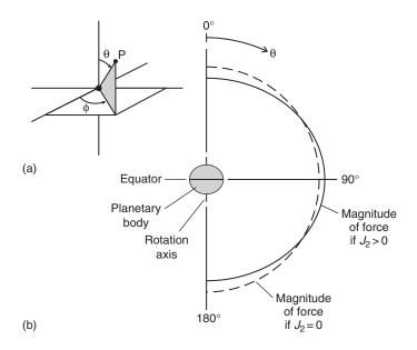
**Figure 4.2** (a) Specifying the position of a point P. (b) The variation of gravitational field with  $\theta$  at a fixed distance r from the centre of a planetary body with  $J_2 = 0$  and  $J_2 > 0$ .
