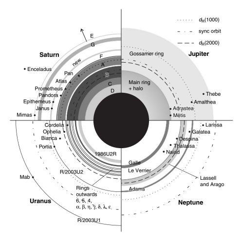
**Figure 2.14** Simplified diagram of the ring systems of the giant planets, scaled so that all four giants are the same radius.  $d_{\rm R}(1000)$  and  $d_{\rm R}(2000)$  are, respectively, the Roche limits of bodies with densities  $1000\,{\rm kg\,m^{-3}}$  and  $2000\,{\rm kg\,m^{-3}}$ . The synchronous orbits are also indicated.
