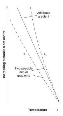
**Figure 4.15** The adiabatic temperature gradient and two possible actual gradients. Note that B has the greatest gradient, because in this context the gradient is the rate of decrease of temperature with increasing distance from the centre.
