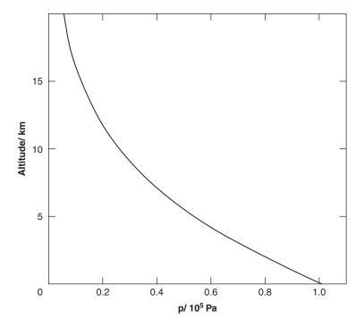
**Figure 9.6** Pressure versus altitude in the Earth's atmosphere.
