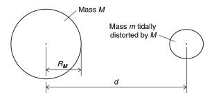
Figure 2.15 Tidal distortion, to illustrate the Roche limit.
