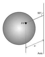
**Figure 4.3** The basis of calculating a moment of inertia.
