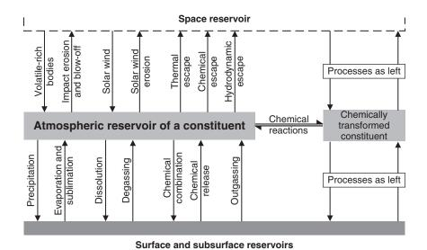
**Figure 9.10** The reservoirs of some atmospheric constituent, and the various types of process by which it can be transferred from one reservoir to another.
