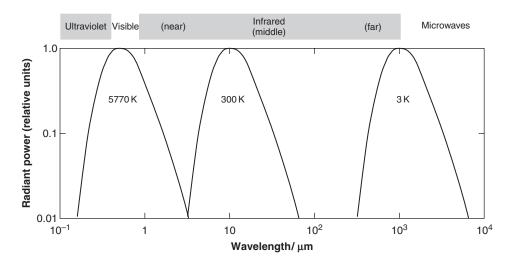
**Figure 4.13** The radiation spectra of ideal thermal sources at various temperatures. Note that the lower temperature spectra have been scaled upwards to a peak radiant power of 1.
