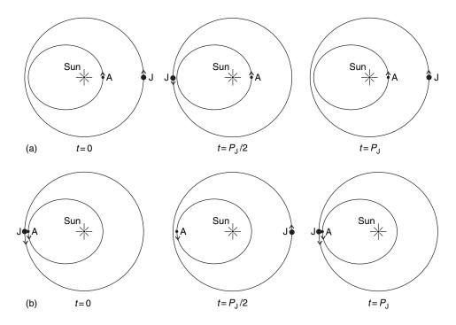
**Figure 1.14** A 2:1 mean motion resonance (mmr) between Jupiter and an asteroid. (a) The perihelion of the asteroid occurs when it is in line between the Sun and Jupiter (probably stable). (b) The aphelion of the asteroid occurs when it is in line between the Sun and Jupiter (probably unstable).
