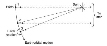
**Figure 1.19** The rotation of the Earth with respect to the Sun and with respect to the distant stars (*not* to scale).
