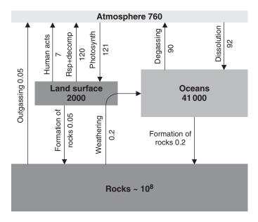
**Figure 10.3** The main features of the Earth's present-day carbon cycle. The size of each reservoir is given in  $10^{12}$  kg of carbon, and the rates of transfer in  $10^{12}$  kg of carbon per year.
