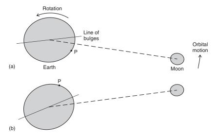
**Figure 4.12** Tides (greatly exaggerated) in the Earth due to the Moon (a) at some instant and (b) about 6 hours later, with the orbital motion of the Moon exaggerated five times. P is fixed to the Earth's surface.
