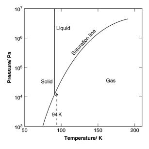
**Figure 10.17** The phase diagram of methane.
