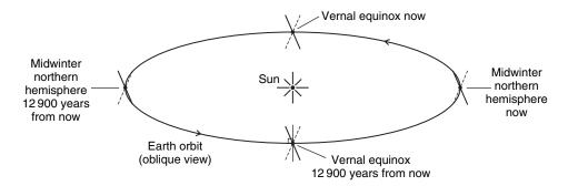
**Figure 1.23** The effect of the precession of the Earth's rotation axis on the position of the equinoxes and solstices. The dashed line is the Earth's rotation axis now, and the solid line the axis 12 900 years from now.
