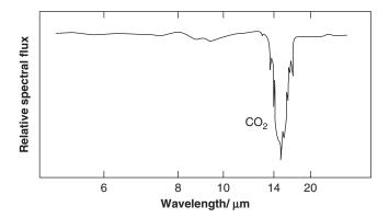
Figure 9.1 Part of the IR spectrum of Mars, with a prominent absorption line due to  $CO_2$ . Note that the smooth shape of the spectral flux from an ideal thermal source at 273 K has been subtracted. (Adapted from C.A.Beichman, JPL Publication, 96-22, (1966))
