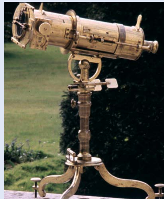
Gregorian reflectors made by Short were in widespread use at the end of the eighteenth century. Apart from a large telescope with a 310mm aperture, Messier used a smaller model similar to the one pictured here.
